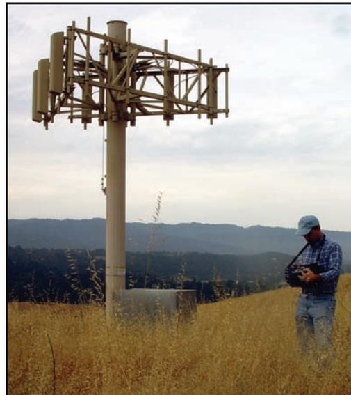
*With capabilities such as precision return loss/ VSWR, cable loss and distance-to-fault (DTF) measurements, the Site Master™ family of analyzers helps field technicians detect problems before they become costly system failures.*
