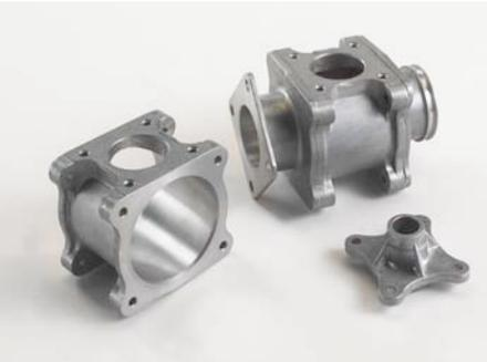
*Valve bodies, pump housings and enclosures of many types can be successfully die cast to save machining time and reduce costs.*
