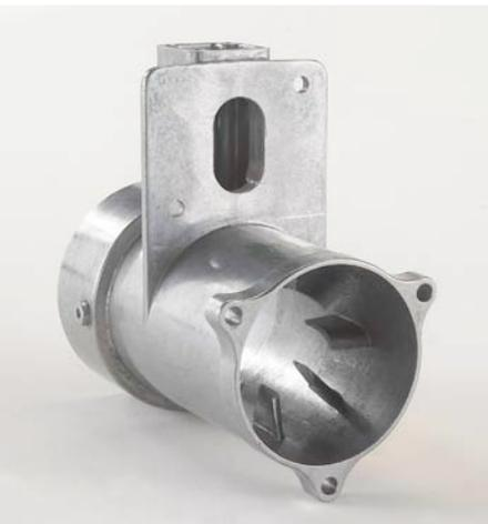
*Die casting can readily produce components with a wall thickness of .060" and even less.*
